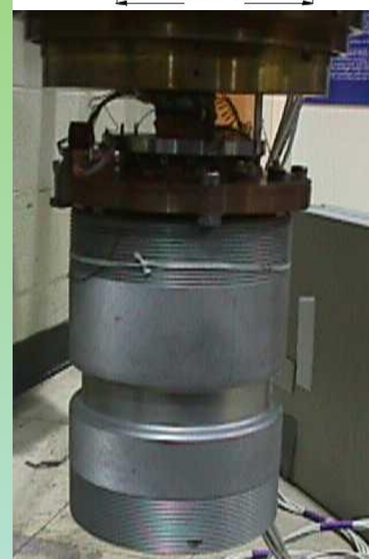
McWhan Clamp Cell schematics and as seen mounted on SD-55 (below)
