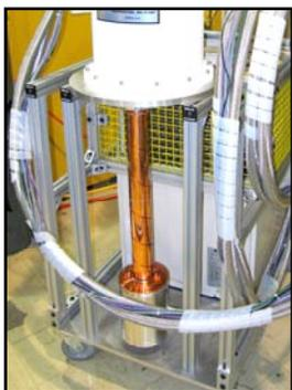
currently take 8 hours to cool to base temperature from 300K and 2.5 hours to warm from base temperature back to 300K. However, while the cryostats can reach 800K, our Aluminum sample cans and heat shields cannot. So for the moment, we must limit temperatures to 700K.
