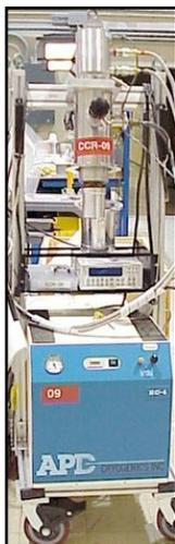
Note that the ARS CCRs are identified by having either blue or blue and white compressors. The Leybold CCRs with orange and black compressors will not be modified; in fact, they will slowly be cycled out of the NCNR.
