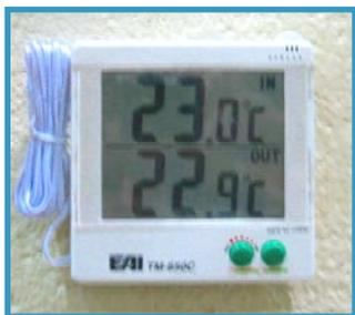
The best way to be assured that the controller is set up correctly and that the sensors are working properly is to check the sensor readings at room temperature **before** an
