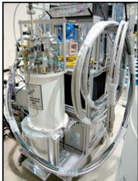
A fresh mix of Top Loading Closed Cycle Refrigerators (TLCCRs) are filtering into the sample environment fleet. We have two short-tailed TLCCRs for general use while others with customized tail sets are dedicated to HFBS, DCS, and FANS. The noticeable asymmetry of the
