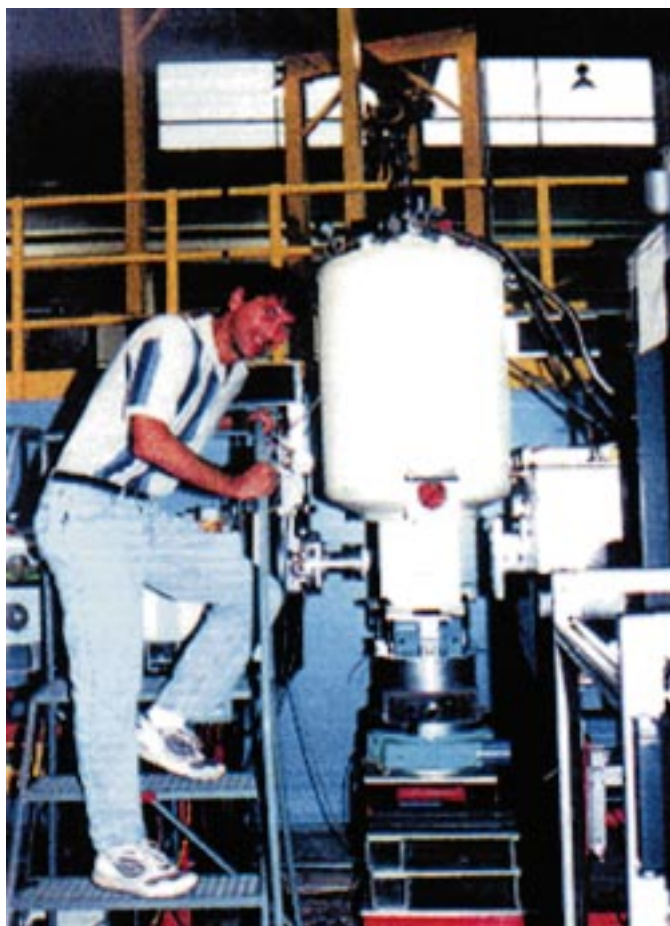
FIGURE 4. John Barker sets up the recently repaired superconducting horizontal field magnet on the NG-7 SANS.
