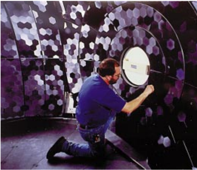
FIGURE 3. Scott Slifer adjusting the analyzer assembly on the HFBS.
