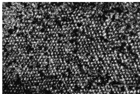
Fig. 5. Transmission electron micrograph of a polymerized dienylyl substituted lipid, cross-linked in a cubic mesophase; scale bar = 100 nm. (Adapted with permission from [98].)
